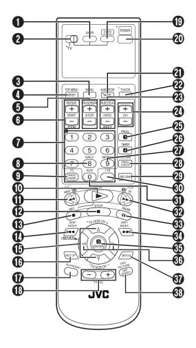
Buttons with a small dot on the left side of the name (**POWER** ( $(\cup)$ ), **TV/VCR**, **TV/VCR CH +/–**, **TV VOL+/–**, **MUTE**) can also be used to operate a JVC's TV after setting the **TV/VCR/DVD** switch to the left.
